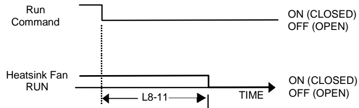
Fig 5.38 Heatsink Cooling Fan Operation Timing Diagram
