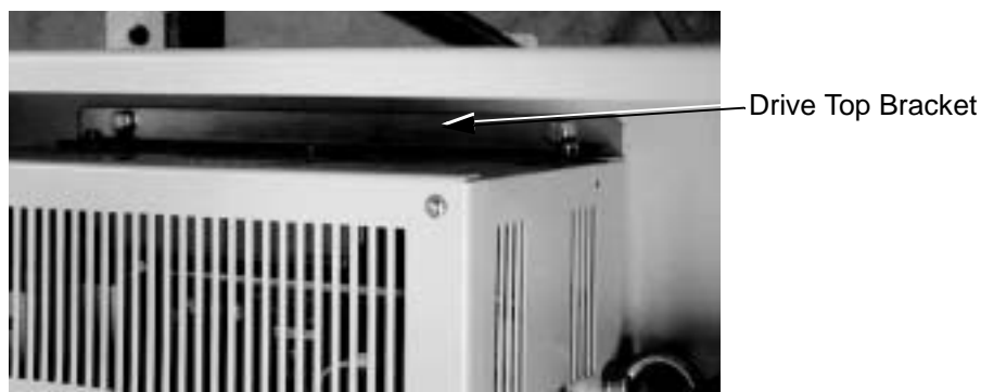
Fig 7.8 Drive Top Mounting Bracket
